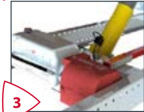
High tipping capacity 7T1 for a 3260 mm tipper (load uniformly distributed)
