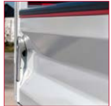
Double safety device and handle incorporated into the sideboard, thus preventing unexpected opening by collision
